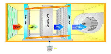
FIGURE 2 – Heat Pipes for Dehumidification
