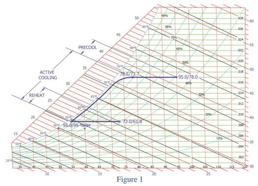
Figure 1 shows the psychrometrics of the wrap around heat pipe installed in an air conditioning system. The upstream heat pipes sensibly precool the air to 78.5DB/73.7WB which then enters the cooling coil. The cooling coil cools and dehumidifies the air to 56.5DB/95%RH/55.0DP. The downstream heat pipe then sensibly reheats the air the same amount to 73DB/61.8WB. The heat pipes then replace 16.5°F of reheat energy and 16.5°F of cooling energy.
